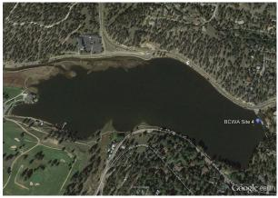
The Evergreen Metropolitan District water plant inlet is near the dam. The raw water is monitored and treated prior to distribution. The plants monitors water pH and turbidity. Periodic samples are taken for metals and other drinking water parameters.
